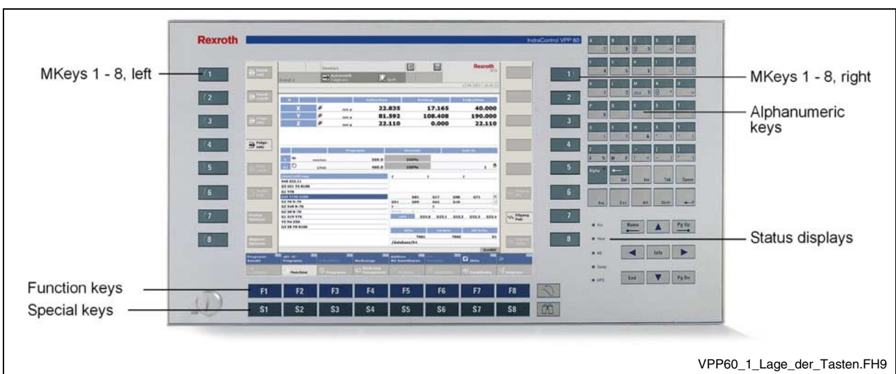
Fig. 6-7: Position of the keys for VPP 60.1
